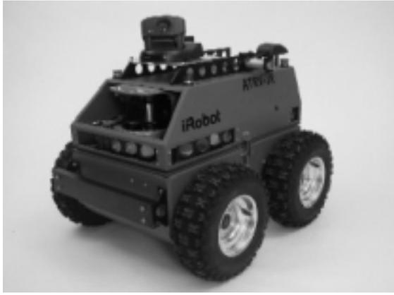
Fig. 1. The ATRV-Jr land robot, fully equipped.
